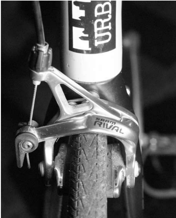
A modern dual pivot front road caliper.
