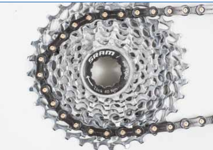
Ramped sprockets allow the chain to mesh smoothly across two cogs, with only two chain links not engaged at roughly the 9 o'clock position.
